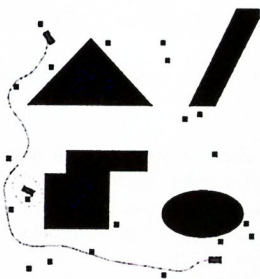
Fig. 6. The reflex actions were not sufficient, the mobile robot collides with a moving obstacle
